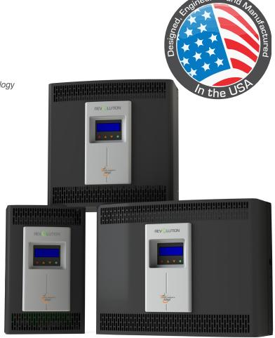
The REVOLUTION Series is an innovative line of ultra-high frequency battery chargers that incorporates cutting edge modular power design that delivers efficiencies greater than 90% throughout the entire charge cycle. As the charge cycle progresses and the output current tapers down, the charger will turn off unneeded modules, allowing the remaining modules to operate at peak efficiency.
